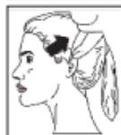
5. While gently pulling the ear, insert the probe snugly into the ear canal (max. 1 sec.) and immediately press the START button. Release the button and wait for the beep sound. This confirms the end of the measurement.
